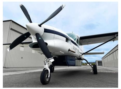
Ampaire's hybrid electric AMP-H570 propulsion system integrated into the Eco Caravan aircraft, at the company's flight test location in Camarillo, California.
