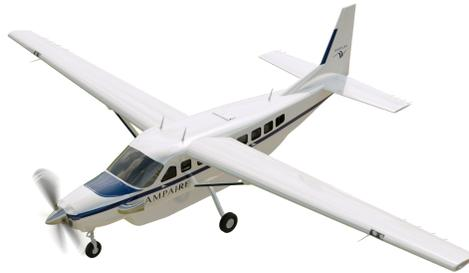
**Oshkosh, WI (July 25, 2022)** Ampaire today announced a key exclusive supplier for the hybrid-electric propulsion system it is developing for its Eco Caravan aircraft, an upgrade to the current Cessna Grand Caravan. Ampaire will use a RED Aircraft AO3 series compression ignition engine rated to 550 hp (405 kW) in an integrated parallel configuration. The RED engine provides the base power and the Ampaire electrical system provides the peak power.
